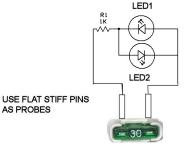
NOTES: THIS FUSE TESTER IS ONLY TO BE USED WITH 12 VOLT CIRCUITS. THIS TESTER TESTS THE FUSE WHILE THE
