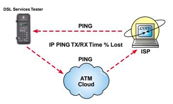
The DSL Services Tester verifies IP layer routing.
