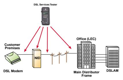
The DSL Services Tester 350+ emulates DSL transceiver-unit modems to confirm DSL physical layer performance.
