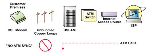
The "NO ATM SYNC" warning indicates an incorrectly provisioned circuit, a DSLAM mapping error, or a misconfigured ATM switch.
